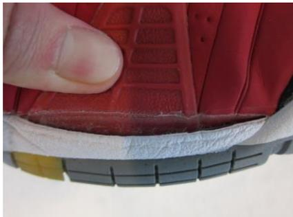
*Parts of the product are not attached correctly*
